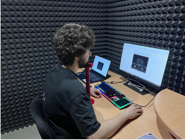
Figure 4: The laboratory setup: the participant at the workstation, the monitor with the stimulus, and the Gazeport GP3 eye-tracker under the lower frame of the monitor. Stable artificial lighting, a room without windows, soundproofing.
